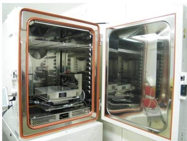
Figure 2 The SGHP 8.2 device located in climate chamber Vötsch VC 0060
