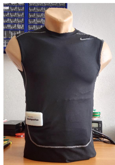
Figure 8 Developed intelligent clothing prototype with processing unit (white box) attached using snap fasteners connected by sewed electro conductive threads
