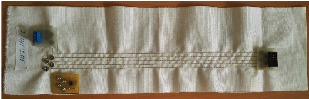
Figure 5 Sample I 2 C bus digital signal transmission – PCB with TMP275 IC, snap fasteners, electro conductive threads
