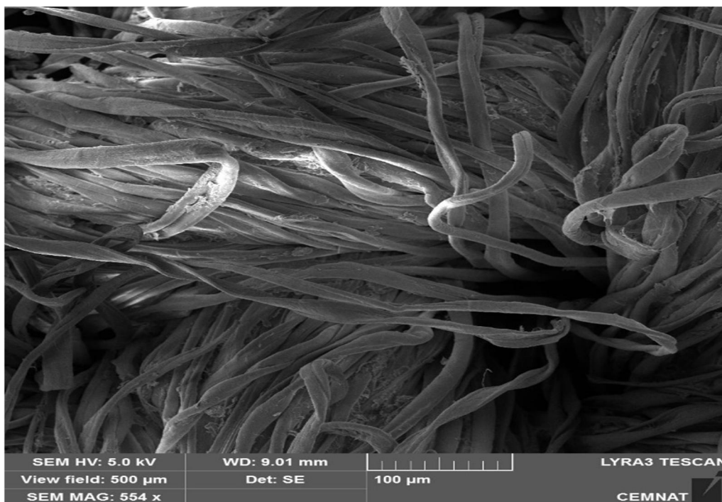
Figure 8 EMS of fiber surface of cotton textile washed with chelating agent no.5
