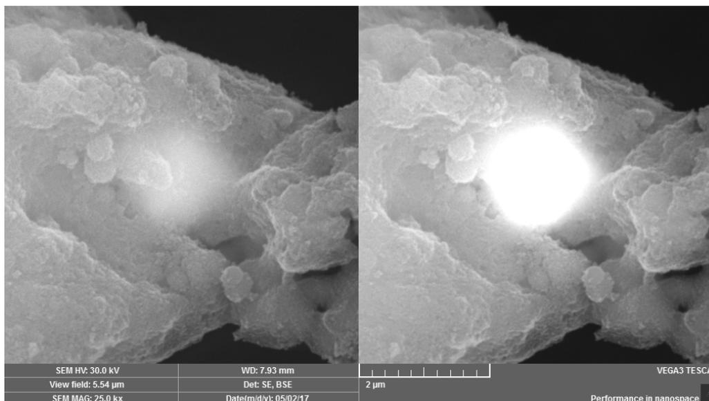
**Figure 3** SEM image of AMB nanoadditive surface with U carrier (PM/B/U sample), magnification: 25000x, left: secondary ray, right: reflected ray
