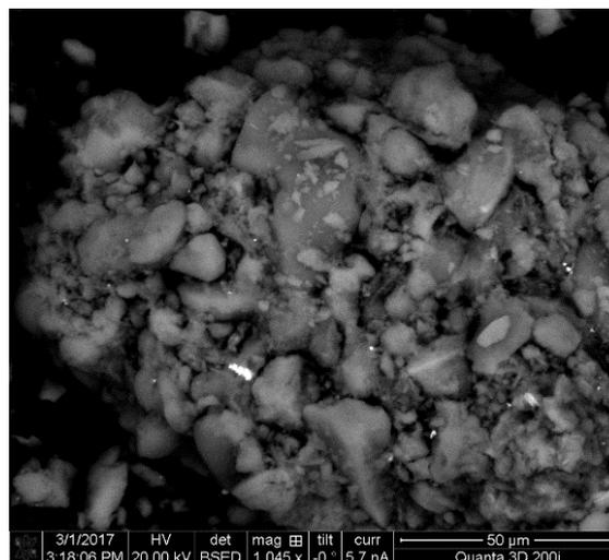
**Figure 1** SEM image of AMB nanoadditive surface with S carrier (PM/B/S sample), magnification 1453x
