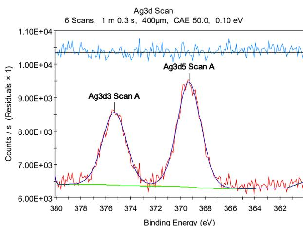
**Figure 4** Graphical record of XPS analysis of the sample PM/B/U with identification of  $\text{Ag}^+$  ion at energetical wavenumber 369.3 eV
