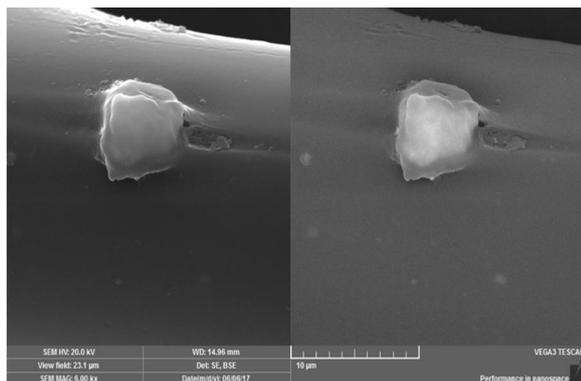
**Figure 5** SEM image of PP fibre surface with a particle of AMB nanoadditive (sample PM/B/U – 10 wt.%, additive concentration 0.75 wt.%), magnification 6000x
