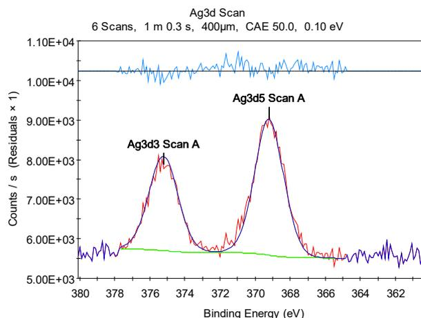
**Figure 2** Graphical record of XPS analysis of PM/B/S sample with identification of Ag<sup>+</sup> ion at energetical wavenumber 369.3 eV
