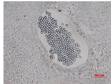
Figure 1b PA single multifilament yarn cross-section
