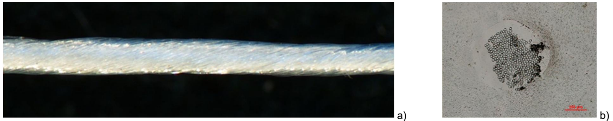
Figure 4 Twisted PES multifilament yarn 2x1110 dtex, Z = 160 \text{ m}^{-1} ; a) longitudinal view; b) cross-section
