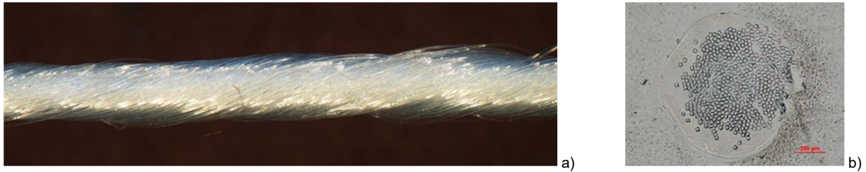
Figure 3 Twisted PA multifilament yarn 2x1880 dtex, Z = 160 \text{ m}^{-1} ; a) longitudinal view; b) cross-section
