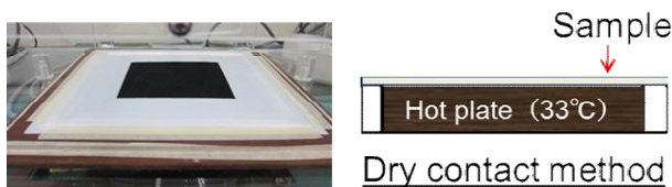
Figure 6 Special type thermal characteristic measuring device (NT-H1: KATOTECH): Thermal resistance
