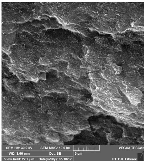
**Figure 4** The homogeneous dispersion of MWCNT in PBT nanocomposites with 5% weight ratio of MWCNT
