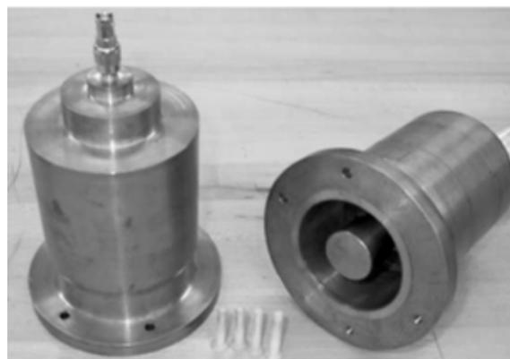
**Figure 2** Coaxial sample holder from company Electro-Metrics Inc. model EM-2107A
