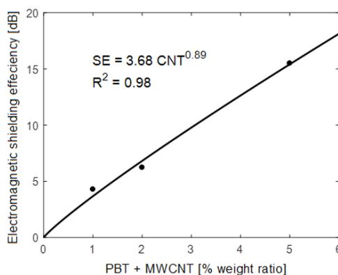
**Figure 5** Dependence of electromagnetic shielding efficiency on MWCNT content in PBT interleaved by power function with its expression
