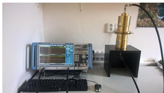
**Figure 3** Electromagnetic shielding efficiency meter with Rhode & Schwarz ZNC3 circuit analyzer
