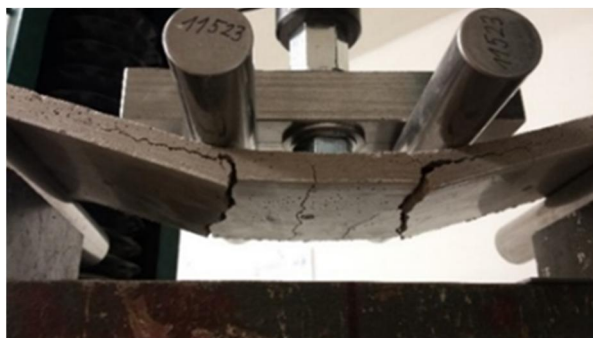
Figure 5 Failure modes of geopolymer composite: a) geopolymer thin plates with one-layer of textile and without addition of BF; b) geopolymer thin plates with addition of 7.5% BF and one-layer of textile
