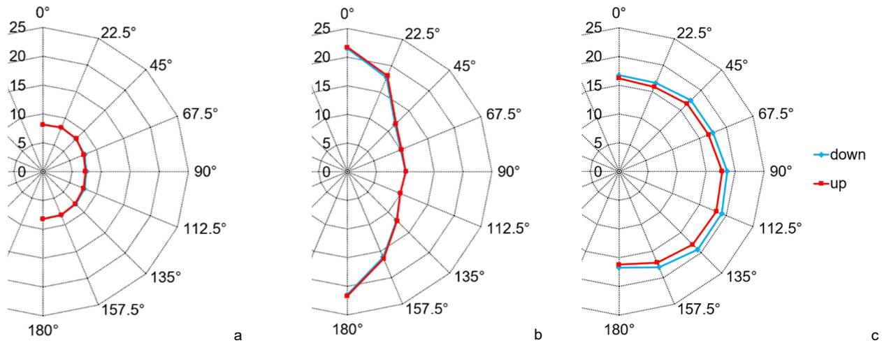
**Figure 6** Polar diagram of bending rigidity  $B$  [ $\text{Nm}^2/\text{m}$ ] at  $+90^\circ$  bending a) Sample 5 b) Sample 6 c) Sample 7
