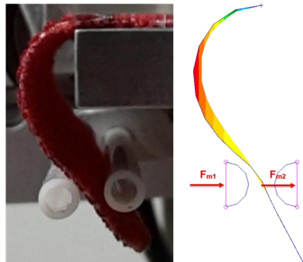
**Figure 7** Comparison of bent shape at bending angle  $+90^\circ$  of sample 6, a) TH-7 test b) FE simulation
