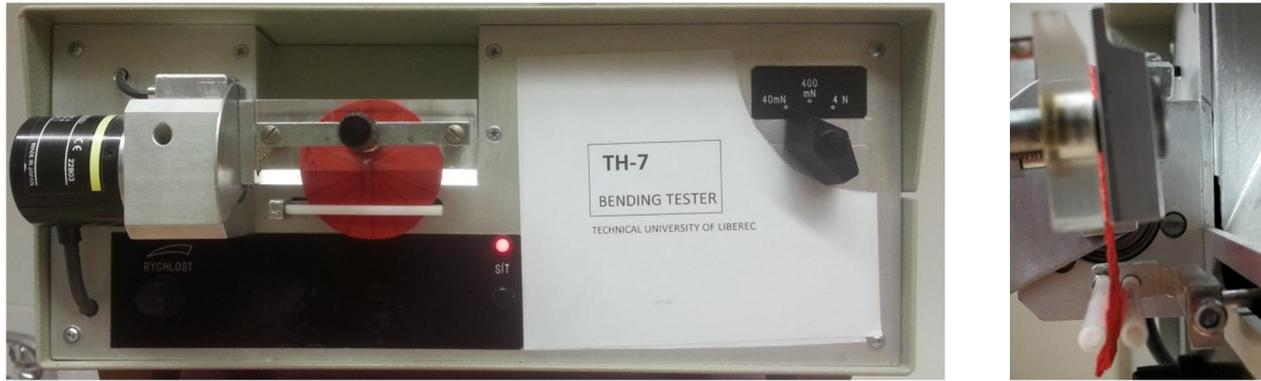
Figure 3 Specimen clamped in the TH-7 bending tester, front and side view
