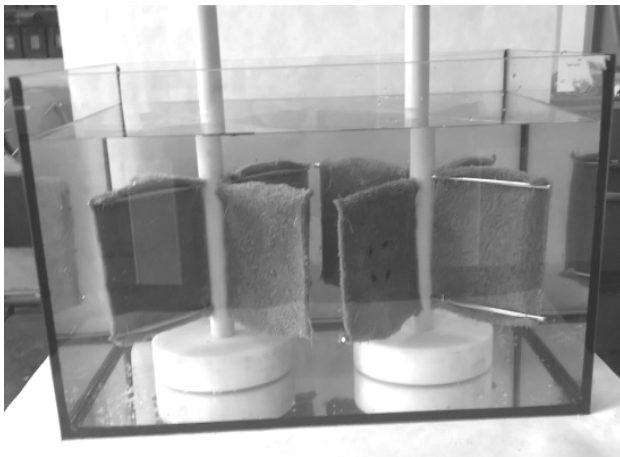
Figure 3 Measurement of absorbency of terry woven fabrics
