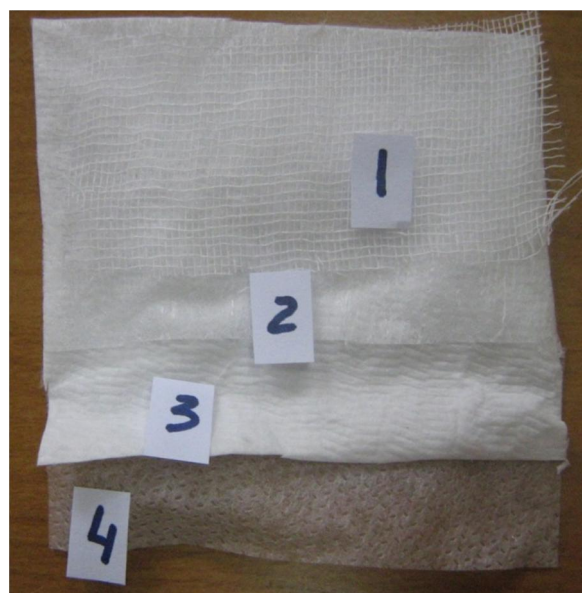
Figure 6 Package of materials for the manufacture of half-masks: 1) inner layer; 2) fine refinement filter; 3) coarse refinement filter; 4) outer frame layer
