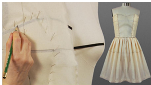
Figure 5a Dressmaker uses pencil, pins and muslin to sculpting the side pattern piece for the dress on the right. The black cotton tape underneath the muslin is used to define the design lines of the dress for the dressmaker to figure out the pattern shape
