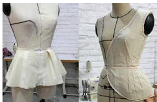
Figure 5b Showing part of the finished muslin shapes of the dress. These 3D muslin shapes will then be converted to 2D pattern pieces on paper for pattern cutting
