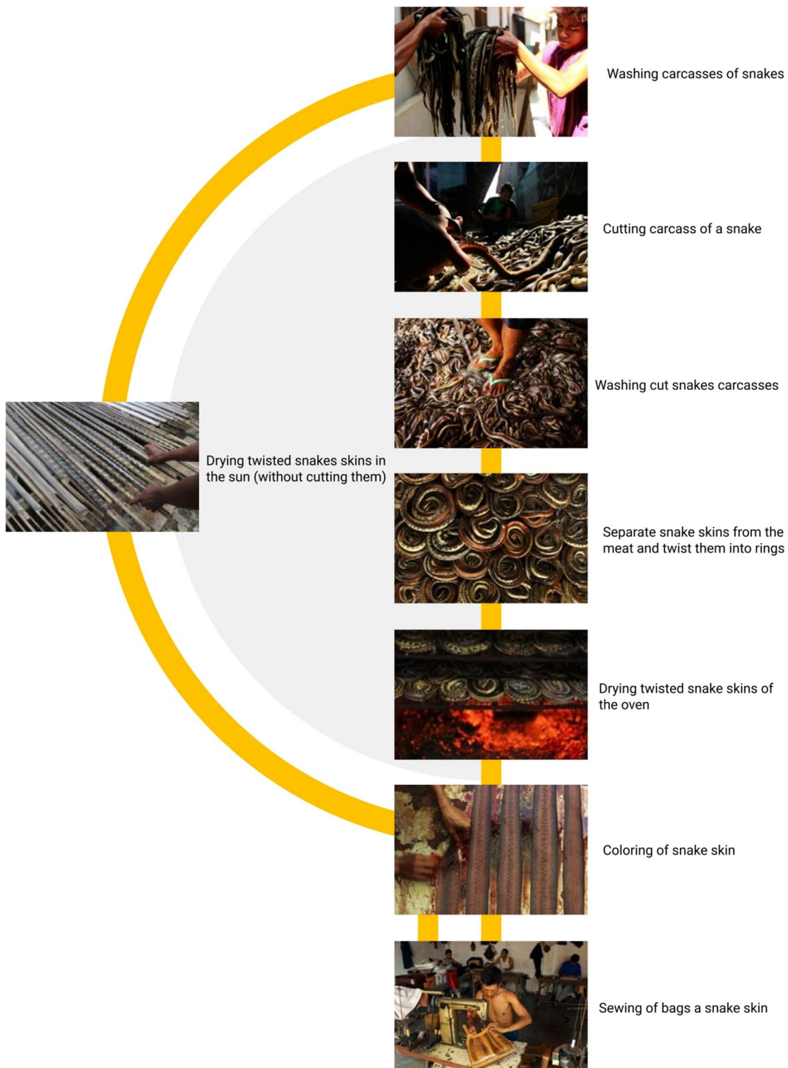
Figure 1 Producing technology of natural snakeskin
