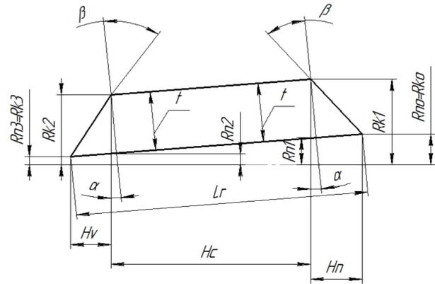
**Figure 1** Geometric parameters of the packing section:  $R_{n0}, R_{n1}, R_{n2}, R_{n3}$  - the inner radii of cones;  $R_{k0}, R_{k1}, R_{k2}, R_{k3}$  - the outer radii of the cones;  $\alpha$  - the angle of the cone of packing;  $\beta$  - the winding angle;  $t$  - is the thickness of the winding body;  $L_r$  - length of layout;  $H_v, H_c, H_n$  - the lengths of the upper, middle and lower sections of the packing respectively.
