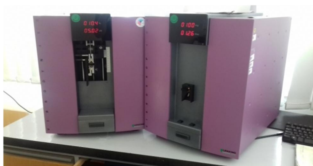
Figure 3 Testing of fiber fineness and strength using VIBROSKOP and VIBRODYN 400
