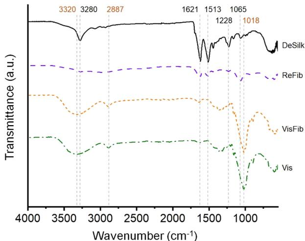
**Figure 5** FT-IR spectra of the samples: (DeSilk) degummed silk fibroin; (ReFib) regenerated silk fibroin in  $\text{Al}_2(\text{SO}_4)_3$  aqueous solution; (Vis) viscose fabric and (VisFib) fibroin treated viscose fabric
