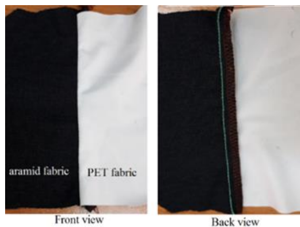
Figure 13 Sewing trial of aramid fabric with polyester fabric
