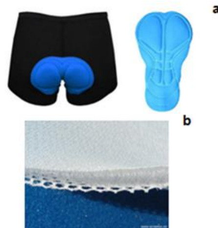
Figure 11 Silicone foam containing cycling short pad vs spacer fabric for soft padding: a) silicon sponge [45], b) spacer fabrics [46]
