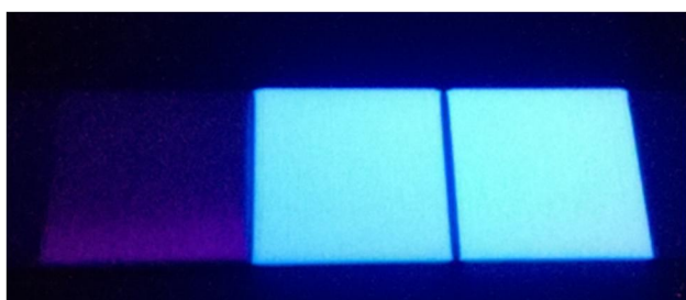
Figure 2 The influence of organic protective photoluminescent pigment with content 0.10 and 0.30 wt.% on the color performance of drawn PLA fibre under a UV lamp
