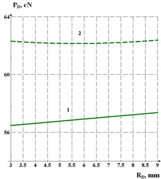
**Figure 8** Graphical dependencies (curves) reflecting influence of guide's radius on yarn tension after the guide for series B: 1 - for the polyethylene multifilament yarn 44 tex; 2 - for the polyamide multifilament yarn 58 tex
