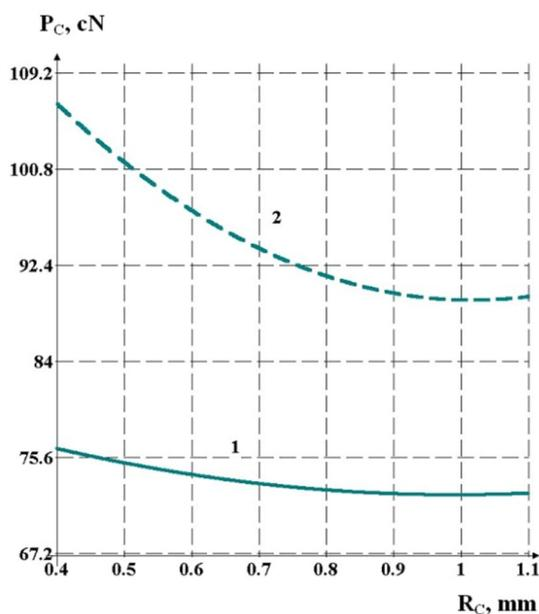
**Figure 9** Graphical dependencies (curves) reflecting influence of guide's radius on yarn tension after the guide for series C: 1 - for the polyethylene multifilament yarn 44 tex; 2 - for the polyamide multifilament yarn 58 tex
