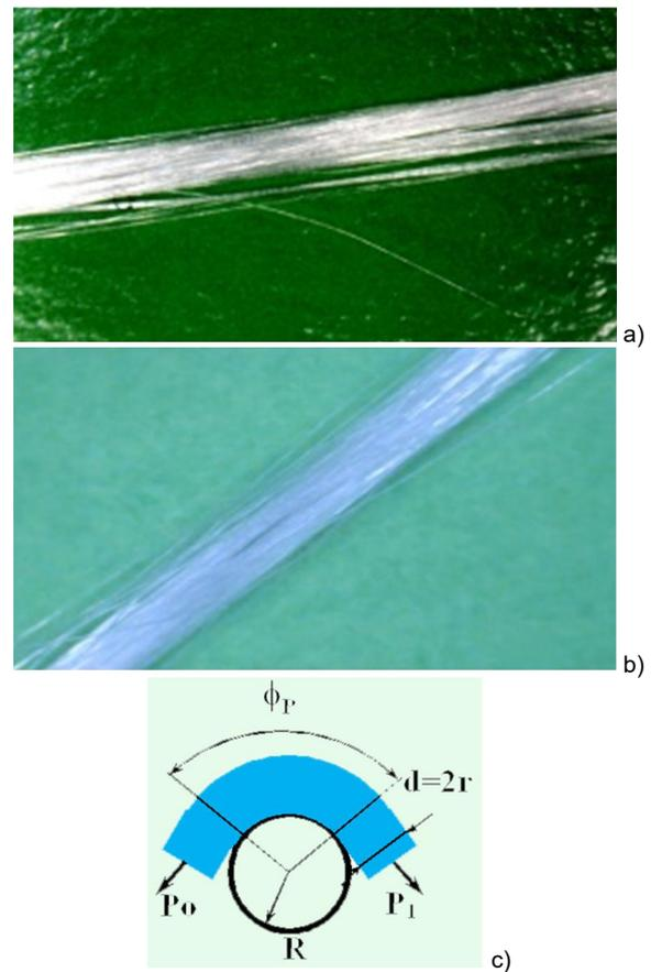
**Figure 4** Multifilament yarns: a) polyethylene multifilament yarn 44 tex; b) polyamide multifilament yarn 58 tex; c) diagram of interaction between a yarn and guide
