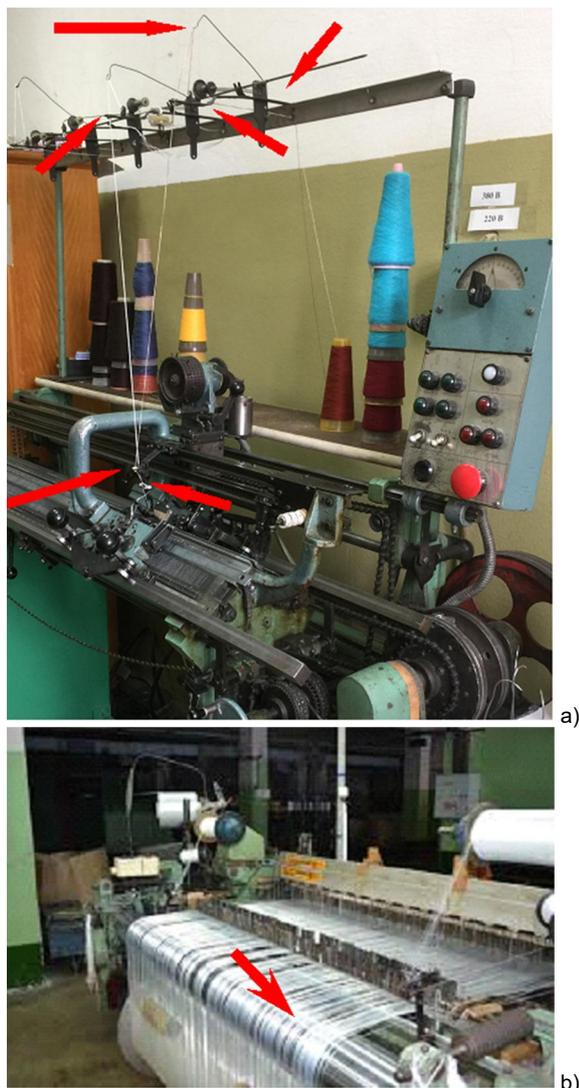
**Figure 2** Threading line in the knitting machine (a) and in the loom (b)
