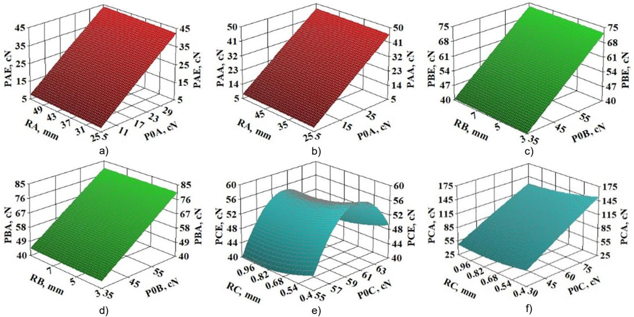
**Figure 6** Response surfaces for series A, B and C created to determine combined influence of the yarn tension before the guide and guide's radius on the yarn tension after the guide: for the polyethylene multifilament yarn 44 tex: a) series A, c) series B, e) series C; for the polyamide multifilament yarn 58 tex: b) series A, d) series B, f) series C
