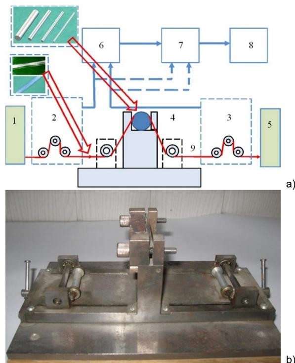
**Figure 5** Scheme of the experimental unit: a) principal scheme: 1 - the yarn threading unit; 2 - metering unit for slack side tension of the yarn; 3 - metering unit for tight side tension of the yarn; 4 - unit for simulation of interaction conditions between the yarn and guides and operative parts of the textile machinery; 5 - yarn receiving unit; 6 - amplifier; 7 - analogue-to-digital converter ADC; 8 - PC; 9 - the yarn; b) central metering unit
