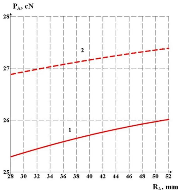
**Figure 7** Graphical dependencies (curves) reflecting influence of guide's radius on yarn tension after the guide for series A: 1 - for the polyethylene multifilament yarn 44 tex; 2 - for the polyamide multifilament yarn 58 tex
