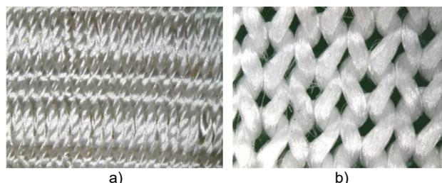
**Figure 1** Industrial fabrics and knits: (a) multilayer industrial fabric of polyamide multifilament yarns; (b) knit of polyethylene multifilament yarns
