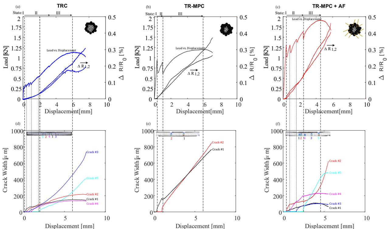
**Figure 3.** Structural and electrical response of TRC, TR-MPC and TR-MPC +AF: (a-c) load vs. displacement and ERC of the carbon rovings, (d-f) crack formation and propagation analysis.
