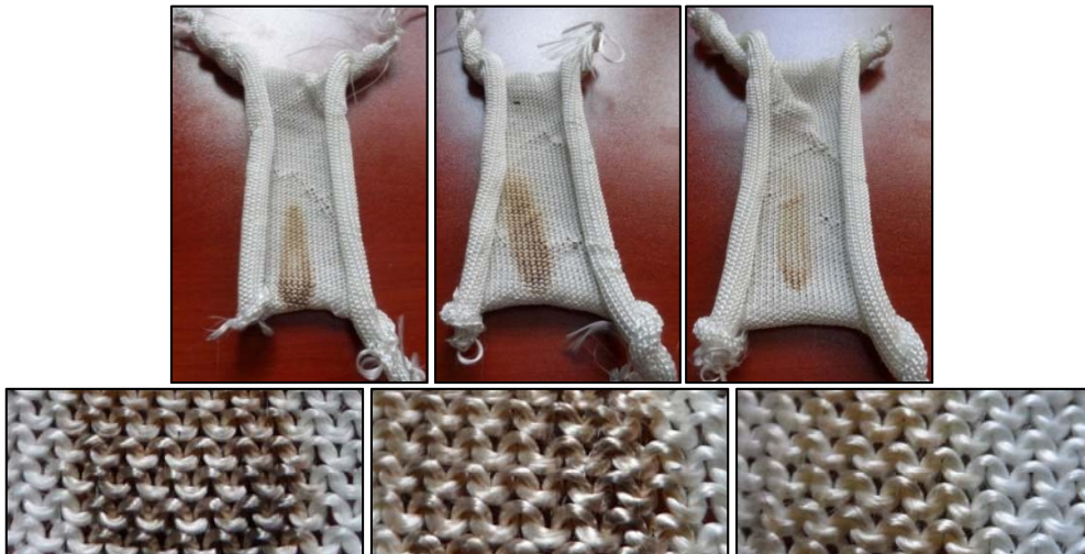
Figure 8. Pictures taken after the burning test of completely glass yarn GG/GG fabric knitted at 4 cam settings.
