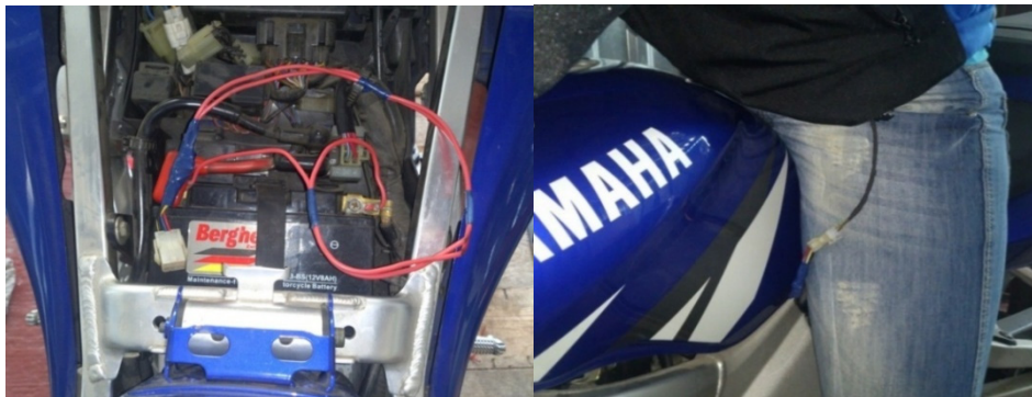
Figure 2. Connection of the electric heating element with a power supply system of the motorcycle.
