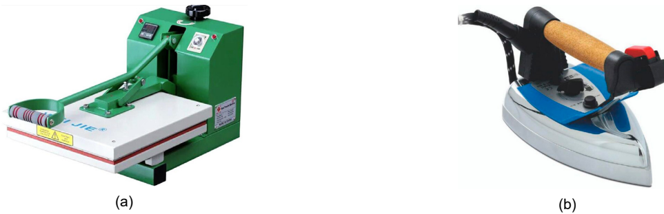
Figure 1. Equipment for transferring a picture to fabric: (a) Thermal printing press Weijie WJ-38, the size of the compression plate: 380×380 mm, power: 3200 W, temperature range: 50-300 °C, timer: 60 s; (b) Steam iron Silter STB-200, weight: 2 kg, power: 800 W.
