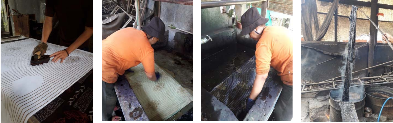
Fig 6. The immersion process of the batik cloth with the mango seed extract.
