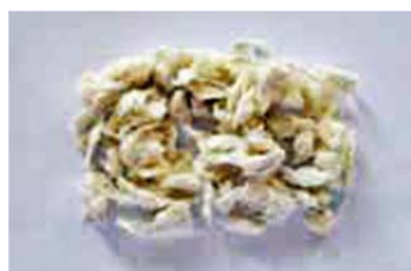
Figure 2. A sample of a cellulose-containing semi-finished product obtained from a shale trust.
