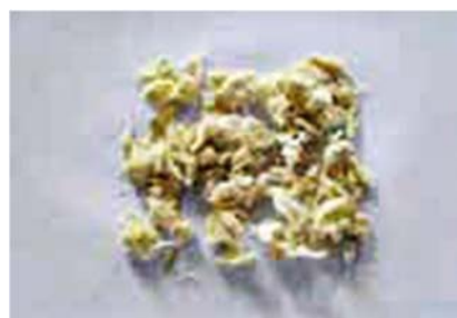
Figure 1. A sample of cellulose-containing semi-finished product obtained from the trust obtained by soaking.
