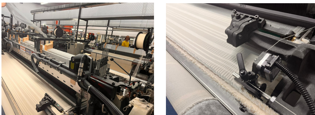
Figure 7. Seersucker fabric production on the machine. (Photograph: Ayçin Asma, 2023).
