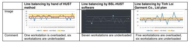
Table 13. Table of comparison of sewing line layout diagram for PL04 product when given the capacity P of Polo-shirt coded PL04.
