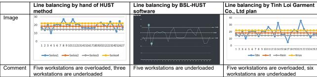
Table 17. Comparison of sewing line layout diagram for Polo-shirt coded PL04 product when given the number of workers N.
