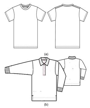
**Figure 1.** Representative images of (a) T-Shirt product - straight shape, rib roll collar, neckline from collar to shoulder, no split, bottom, and sleeve-hem sewing dividing seams with two parallel lines and (b) Polo-Shirt product - Bottom down collar by rib, not neckline; collar panel deviates; long sleeves by rib-knit cuff; split, bottom sewing one diving seam.
