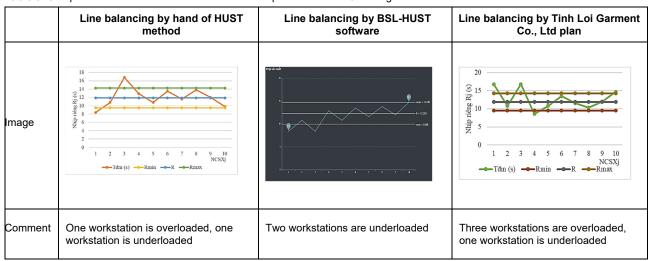
Table 9. Comparison of the sewing line layout diagram for T-shirt product coded T07 when given the number of workers N.
