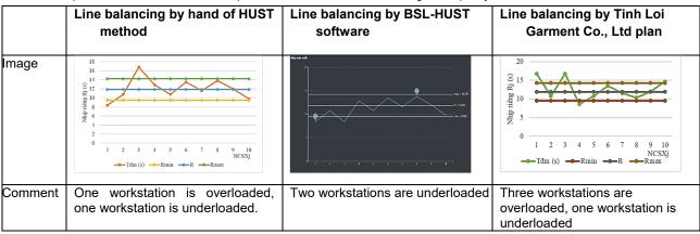
**Table 5.** Comparison of the sewing line layout diagram for T-shirt coded T07 product with the given capacity P.
