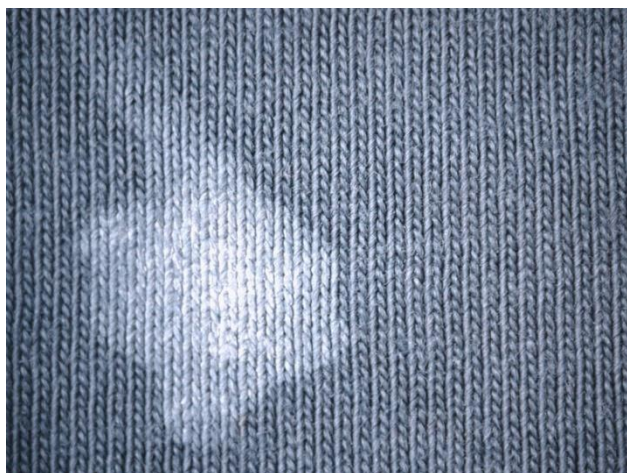
Figure 1. Paint stain on cotton knitted fabric magnified 10x.
