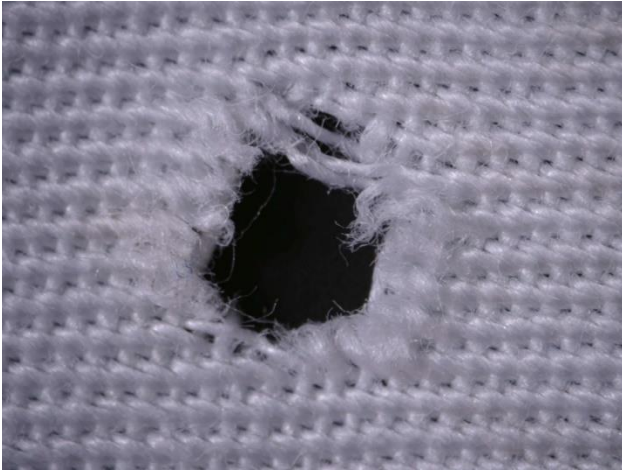
Figure 5. Mechanically damaged cotton fabric - perforations, suitable for repair, enlarged 25x.
