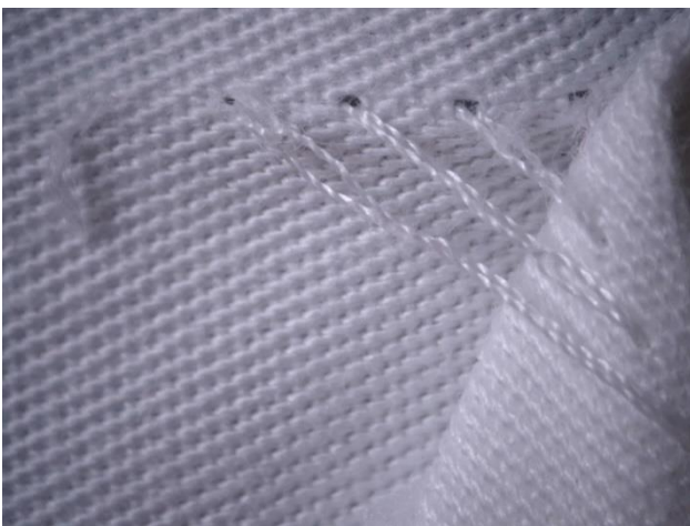
Figure 6. Mechanically damaged cotton fabric - loose pocket, suitable for repair, enlarged 15x.
