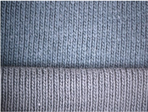
Figure 3. Colour change of cotton knitted fabric due to light and humidity (unexposed on top, exposed knitted fabric on bottom), magnified 12x.
