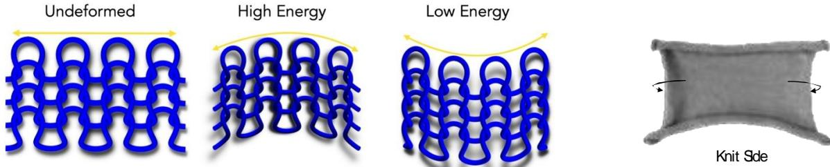
**Figure 9.** (Left) Generalized energy for two knit structure deformation modes. (Right) Natural curling of a single Jersey knitted fabric.
