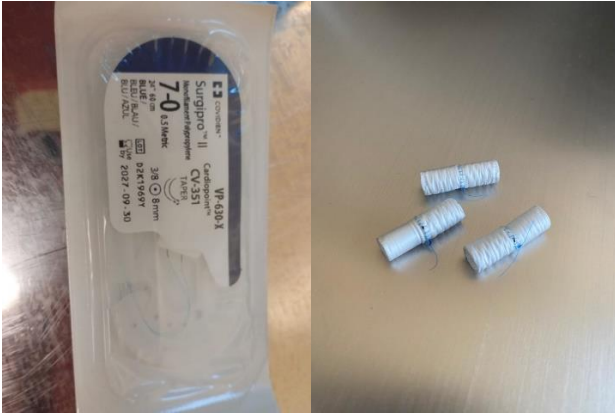
Figure 1. Images of the polypropylene thread used for stitching and the surfaces sewn with continuous stitching.
