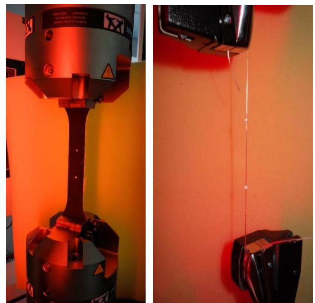
Figure 3. Tensile test of fabric skin and pile yarns using a universal testing machine.
