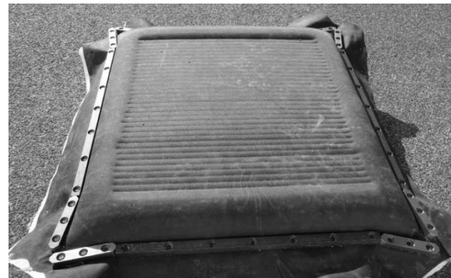
Figure 8. The 3D distance fabric panel during the safety test. In the center there are visible deflections of the skin between binding points that were measured by a laser scanner.
