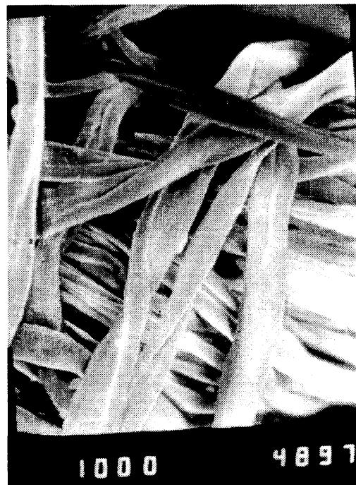
**Fig. 9** SEM photograph of blended fabric of viscose/cotton viscose on check side
