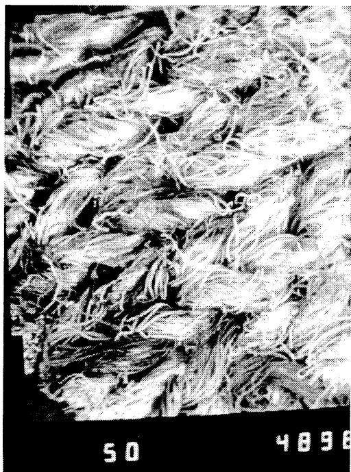
Fig. 3 SEM photograph of integrated fabric of PP/cotton cotton check side
