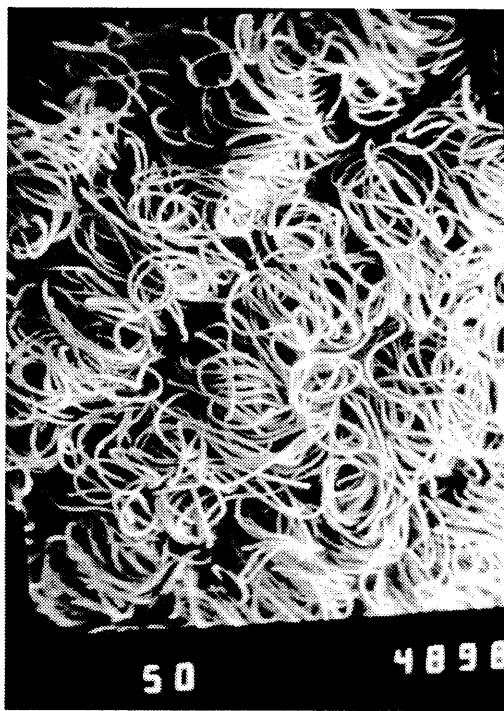
Fig. 4 SEM photograph of integrated fabric of PP/cotton PP loop backing
