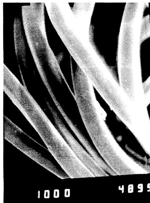
**Fig. 10** SEM photograph of PP fibers
