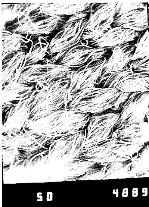
**Fig. 7** SEM photograph of blended fabric of PP/cotton PP fibers on check side
