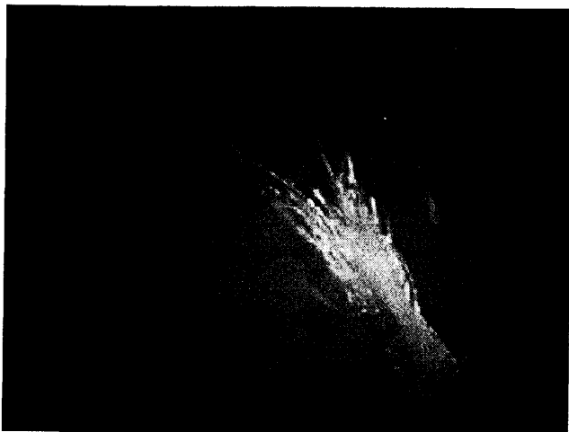
Fig. 4.5. Intentionally broken yarn – fibres also are broken.
