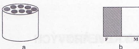
Fig. 1 The linear composite Kevlar epoxy resin (a), corresponding mechanical two- phase model (b).
