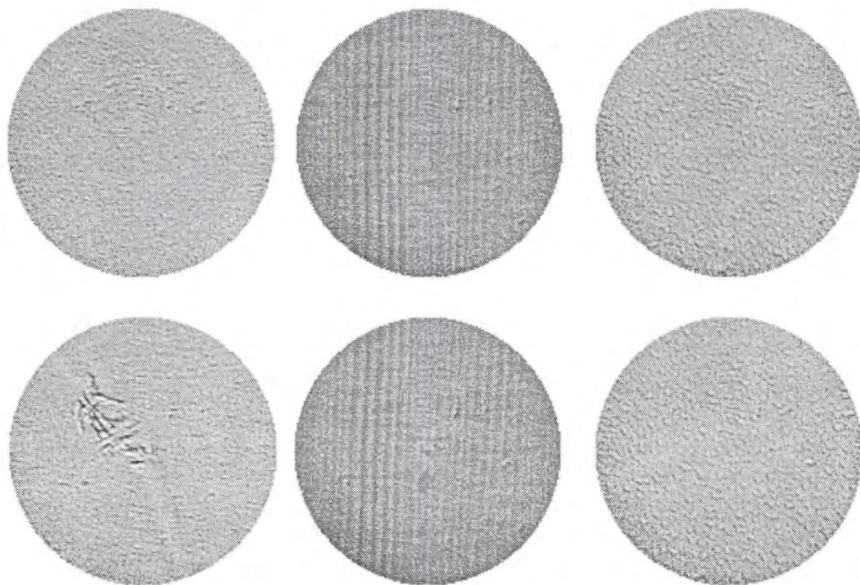
Fig. 10 Samples of tested BOPP foils wit and without defects
