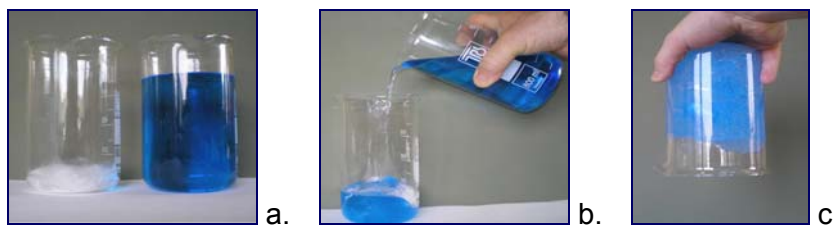
Figure 2 Proof of absorptivity of superabsorbing fibres: a) left: 100% superabsorbing fibre, right: distilled water; b) gradual addition of distilled water to the superabsorbing fibre; c) superabsorbing fibre after absorption of distilled water
