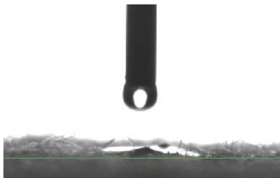
**Obr. 10** Kvapka vody na neupravenej tkanine PES/ba 50/50%
