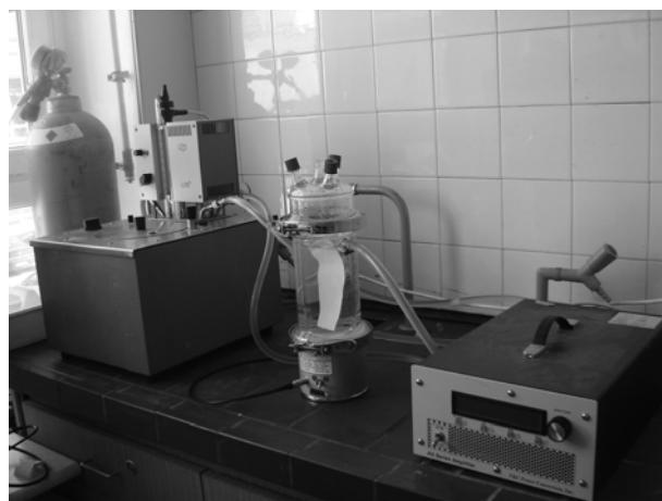
**Figure 1** High frequency ultrasound equipment (University of Maribor)
