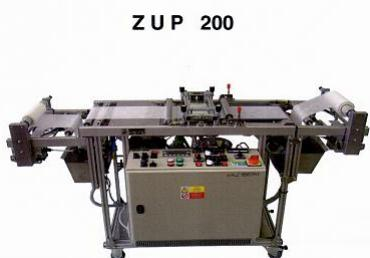
**Figure 1** ZUP 200 Laboratory equipment for Application of low-temperature plasma under atmospheric pressure
