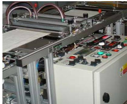
**Figure 2** Plasma treatment of a woven fabric made of 100 % cotton.
