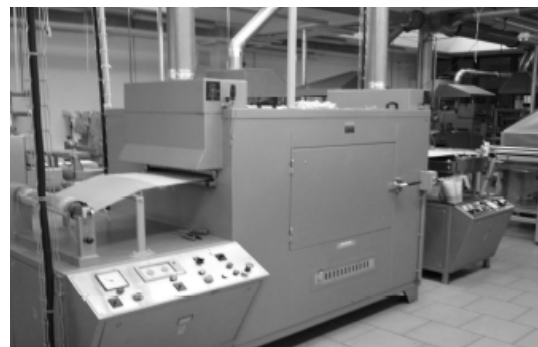
Figure 3 Werner Mathis AG (CH-8155) coating machine with dryer
