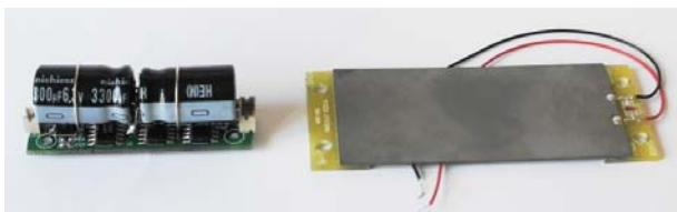
**Figure 2** Piezoelectric element with energy harvesting circuit
