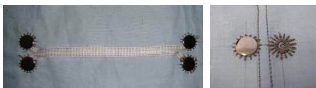
**Figure 4** Conductive trajectory Gibbon and embroidered with conductive ring replacing buttons
