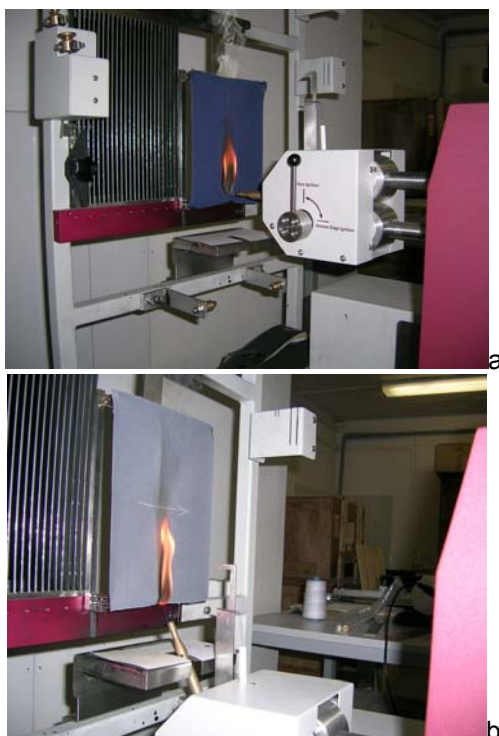
Figure 5 The SDL Atlas M233B AutoFlam tool - a) effects of a flame applied to the surface & b) effects of a flame applied to the edge
