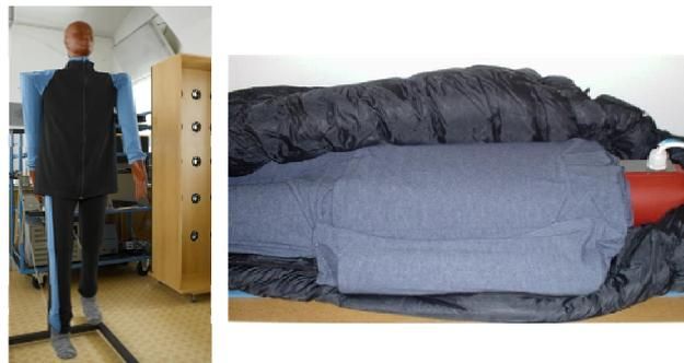
**Figure 1** Manikin according to EN ISO 15 831 [3] (left), manikin according to EN 13 537 [2]
