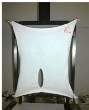
**Figure 3** Vertical flammability test, limited flame propagation
