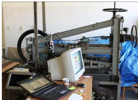
**Figure 1** Static adhesor for experiments bicycle and car tires
