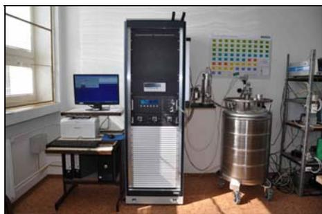
**Figure 2** Experimental equipment for dc electrical conductivity measurement
