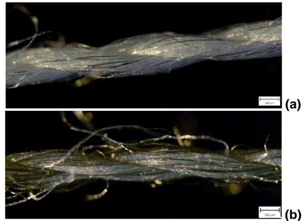
**Figure 1** Microscopic images of two ply hybrid yarns containing (a) 15%, (b) 60% of conductive component
