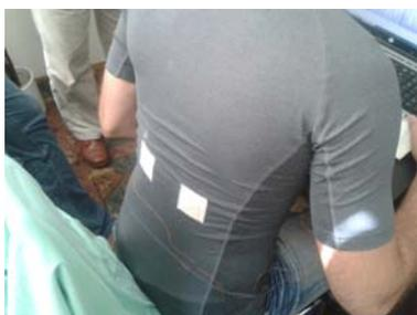
**Figure 1** Position of the active textile electrodes on the first prototype of smart T-shirt
