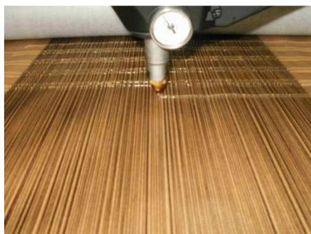
**Figure 3** Prototype machine for manufacturing of the planar fabric – the mobile head and the application of polymer melt on longitudinal threads
