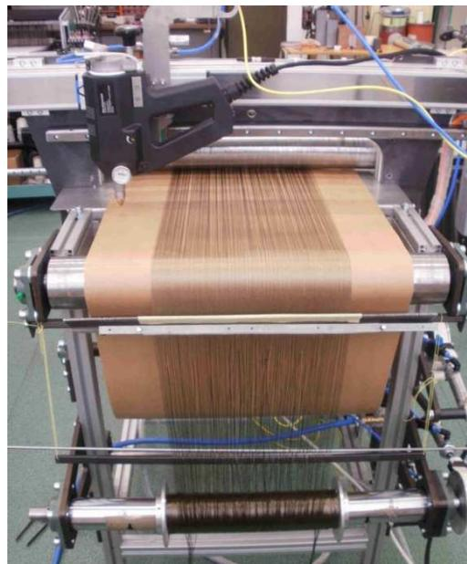
**Figure 2** Prototype machine for manufacturing of the planar fabric
