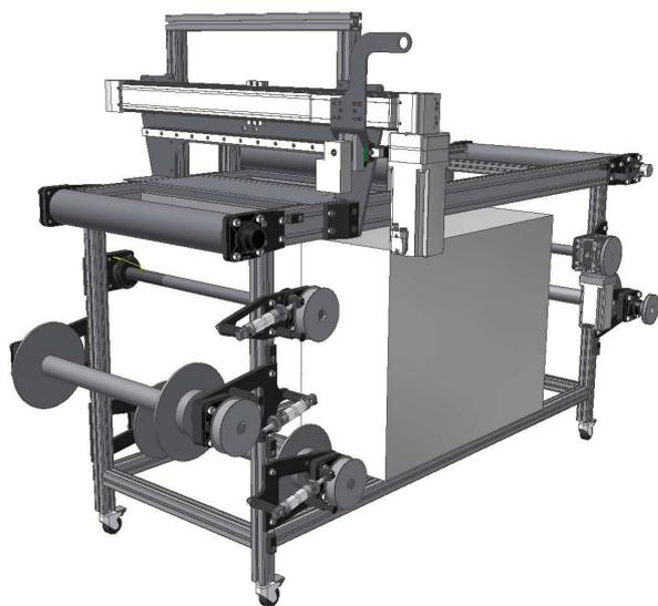
**Figure 1** 3D prototype model of technology for manufacturing of planar textile fabrics bonded by the perpendicular lying of polymer melt
