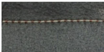
Figure 9 Bobbin thread pulled towards the face of the fabric layer
