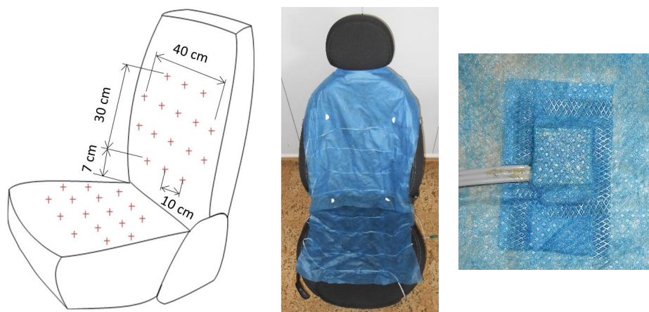
Figure 1 Illustration of measurement of thermal and humidity field by sensor sheet, detail of one sensor
