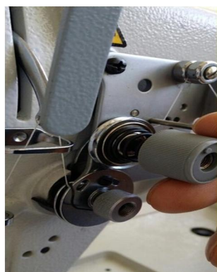
Figure 3 Upper thread tension adjustments
