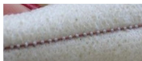
Figure 8 Upper thread pulled towards the bobbin thread
