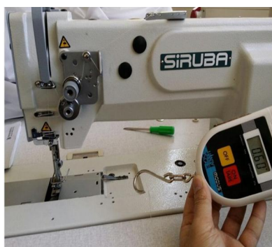
Figure 2 Thread tension measuring device
