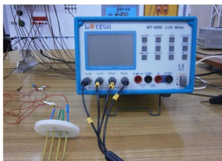
Figure 2 Measuring bridge for testing the resistance of the agar gel and the polyacrylamide gel
