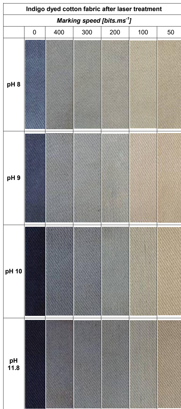
Figure 6 The photos of Indigo dyed cotton samples after laser treatment at various values of marking speed of laser beam
