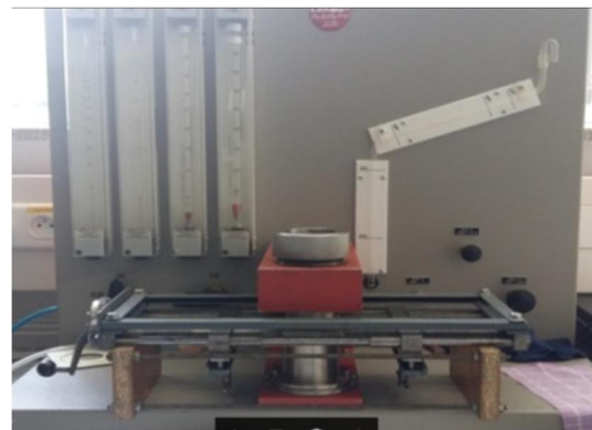
Figure 4 Air permeability measurements (front view)
