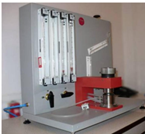
Figure 4 Air permeability SDL M021S
