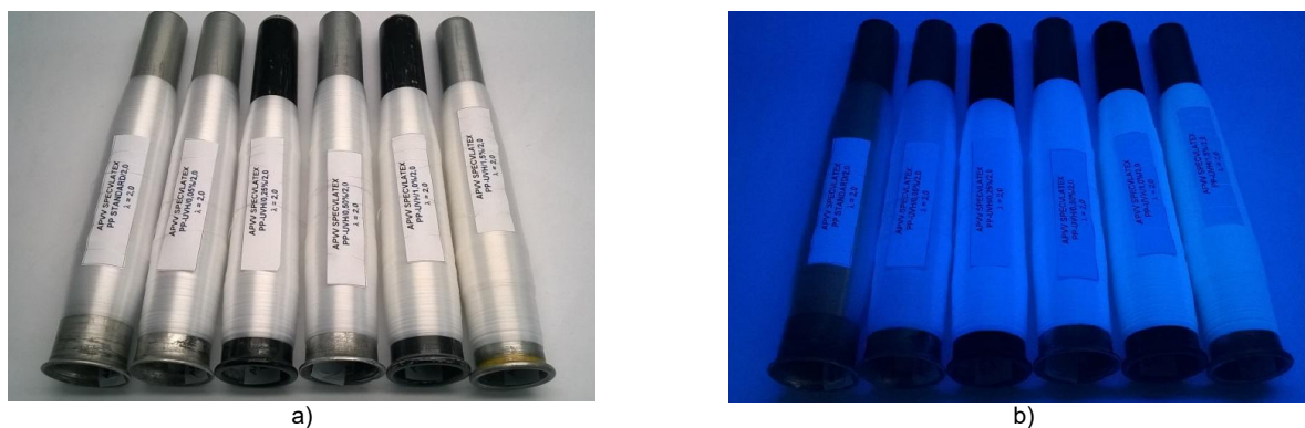
Figure 2 The influence of modified nanofiller M-HNT with a content 0.05; 0.25; 0.50; 1.00 and 1.50 wt.% on the color performance of drawn nanocomposite PP fibres compared with unmodified PP fibre (first from the left) under daylight D65 (a) and under a UV lamp (b)
