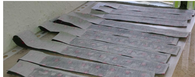
Figure 1 Textile strips, glued with different adhesives, drying at room temperature
