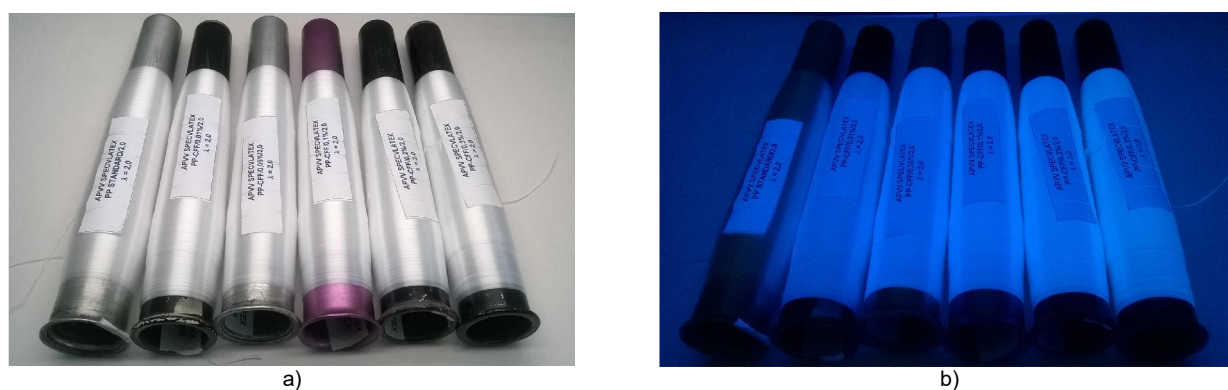
Figure 4 The influence of photoluminescent pigment A with content 0.01; 0.05; 0.10; 0.20 and 0.30 wt. % on the color performance of drawn PP/A modified fibres compared with unmodified PP fibre (first from the left) under daylight D65 (a) and under a UV lamp (b)
