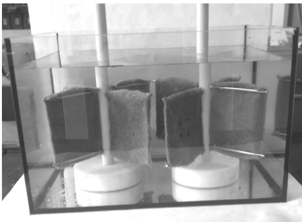
Figure 3 Measurement of absorbency of terry woven fabrics
