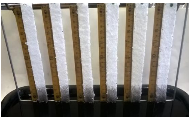
Figure 4 Measurement of wicking of terry woven fabrics
