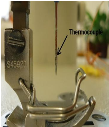
Figure 3 Thermocouple inserted inside needle groove
