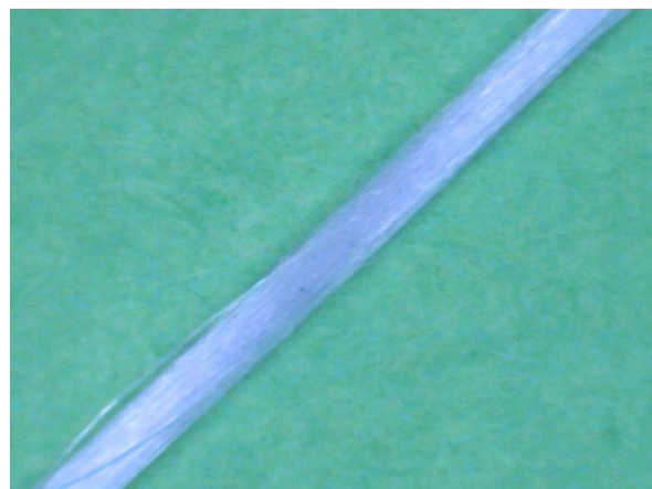
Figure 6 Diagram of polyamide filament yarn 29 tex consisting of 80 filaments, flat twist Kr=400 twists/meter, the nominal diameter d=2r=0.200 mm, the bending modulus B=4.0 \cdot 10^{-2} cN/mm 2
