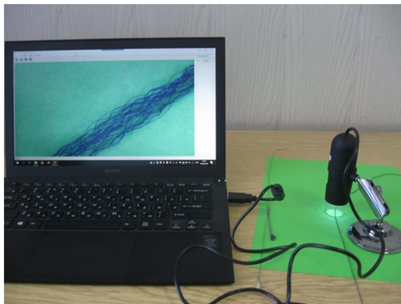
Figure 11 Set-up to determine the radii of the guide way and polyamide filament yarns
