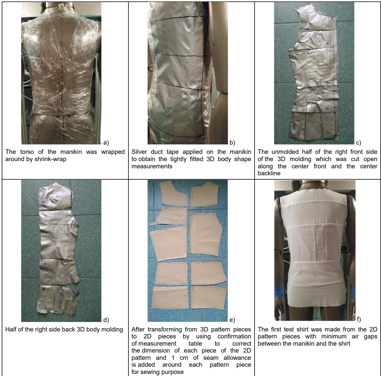
Figure 2 The procedures of the molding method for the torso pattern development
