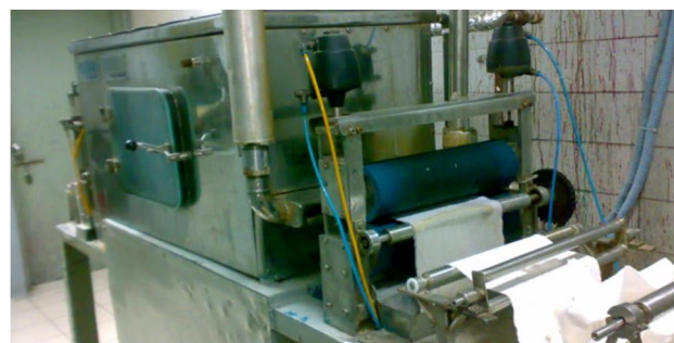
Figure 5 Sample dyeing process in pad dye pad steam machine
