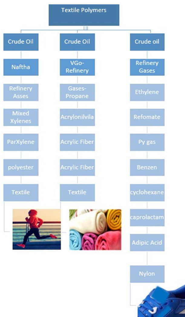
Figure 2 Production stages of textile polymers in Saudi Arabia petrochemical factories
